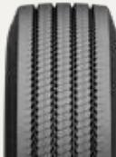
Winter tread with excellent wearing resistance. Suitable for all axles, optimal for short and medium haul trucks and buses. Effective siping and siping activators enhance the grip also in demanding winter conditions. With its cap/base structure, the tire installed in autumn will offer good driving properties also in the next summer.
