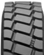
A traction tread designed for off-road use and short transfers in special vehicles such as wheel loaders and dumpers. Special rubber compound guarantees a unique tear and puncture resistance, and the tread has a large block structure with excellent self-cleaning and grip. Noktop 86 is not recommended for long-distance transport during the summer.
