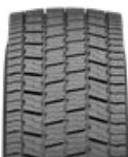
Durable winter traction tread for long haul transport on main roads. Its strong siping provides good grip and traction properties in every weather. Tread design and rubber compound provide excellent mileage.
