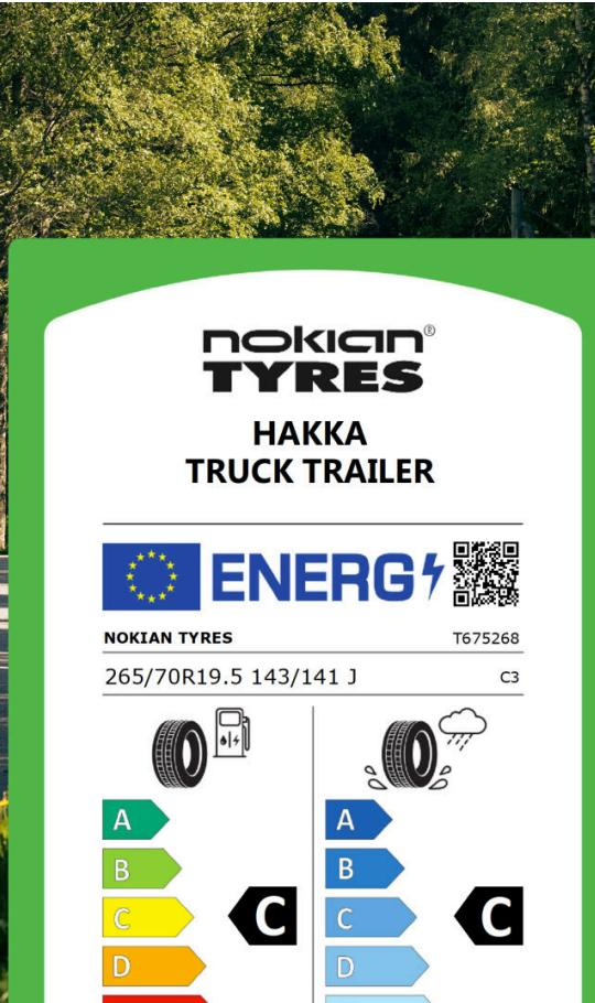
EU tire labelling became mandatory for truck and bus tires in 2021. The labels show important tire properties such as **grip**, **fuel efficiency** and **noise level** at a glance, making it easy to choose a safer, more ecofriendly tire.
