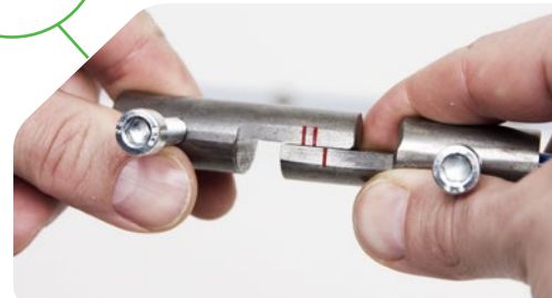
Mandrel gauge for rim circumference measurement
