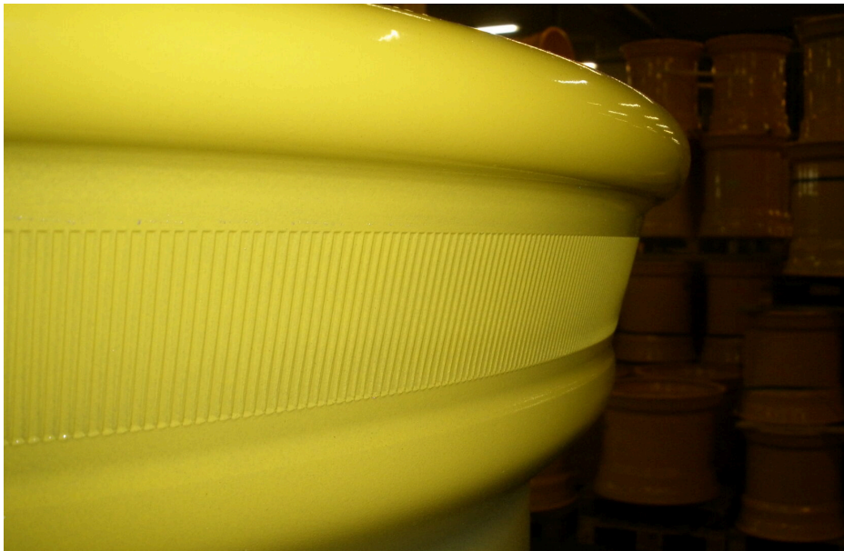
Knurling for tire slippage on rim prevention
