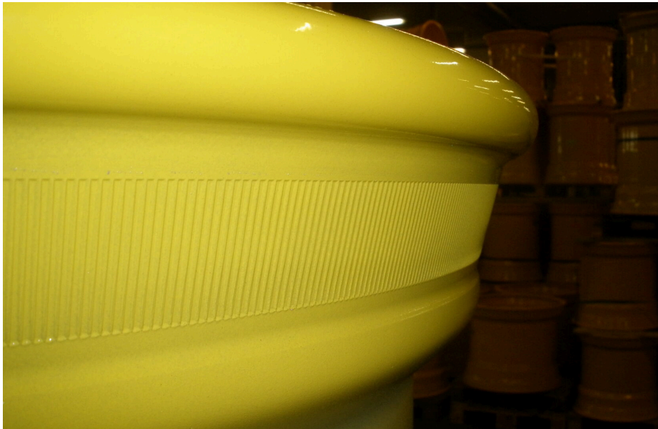
Knurling for tire slippage on rim prevention
