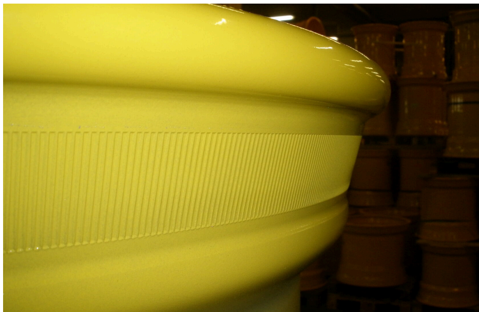
Knurling for tire slippage on rim prevention
