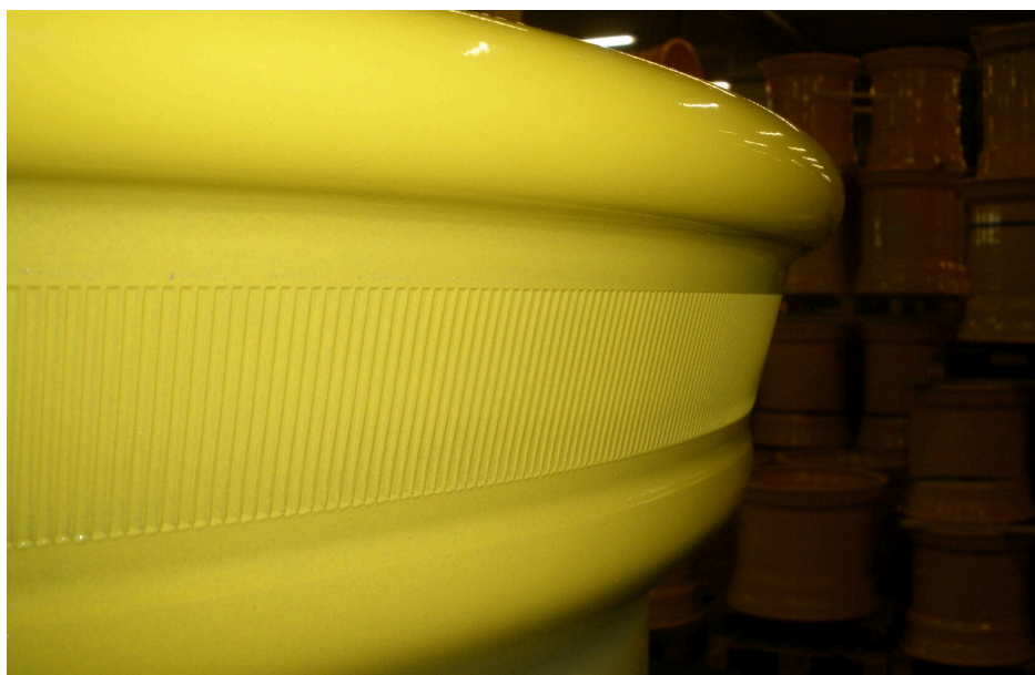
Knurling for tire slippage on rim prevention
