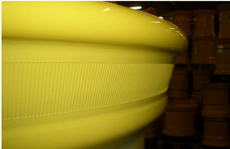
Knurling for tire slippage on rim prevention
