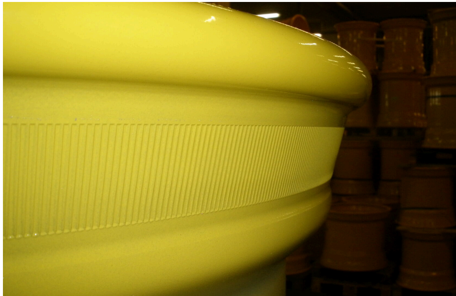
Knurling for tire slippage on rim prevention
