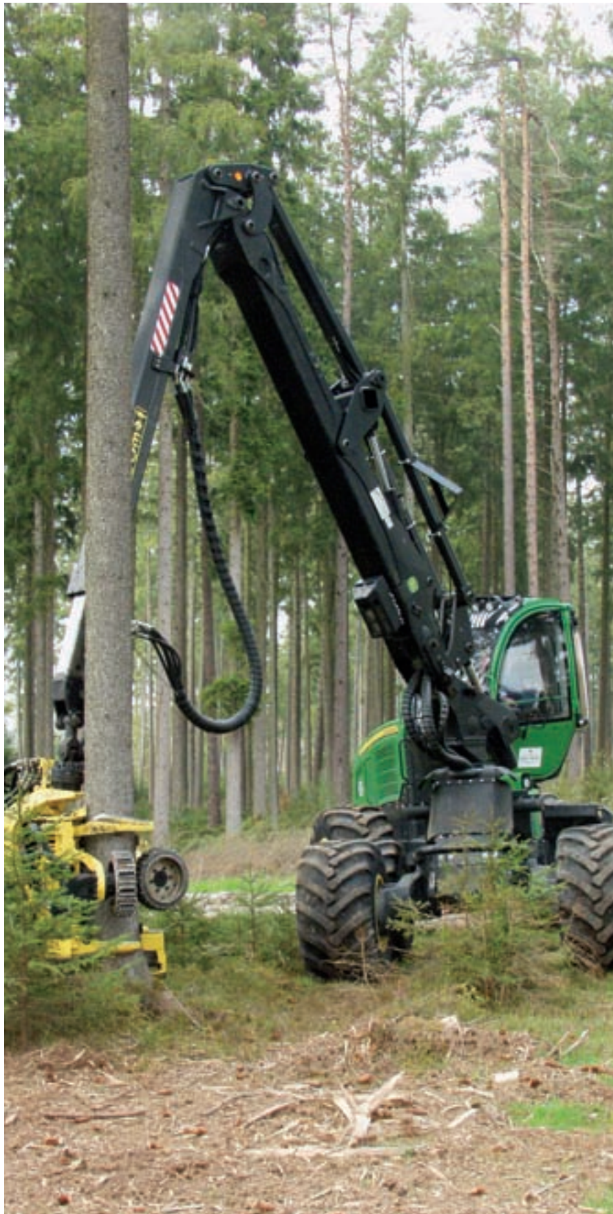
Wide base tyres offer good stability of the machine when cutting heavy trees.
