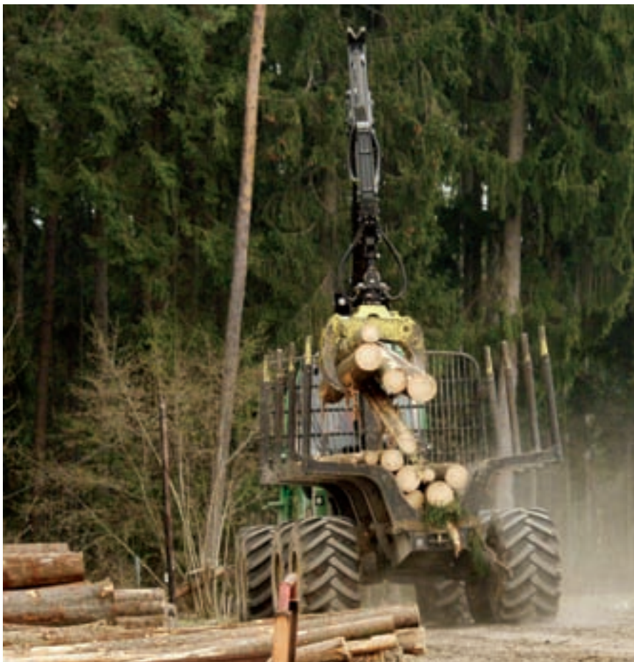
At the woodyard of the Castell holding: The forwarder brings timber for temporary storage.
