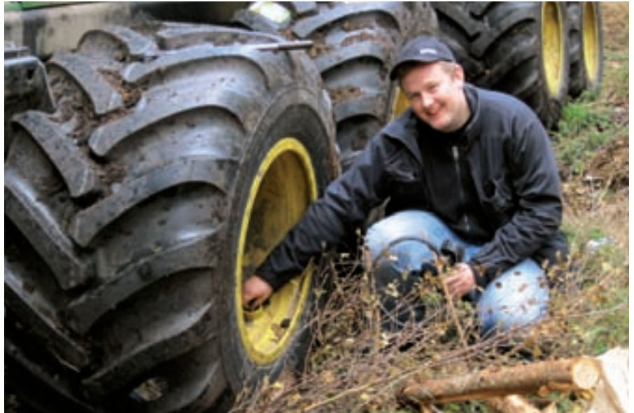
Teemu Vainionpää checks the tyre pressure of Nokian Forest Rider in John Deere 1110D.
